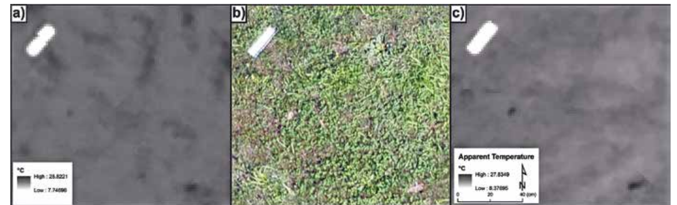
Figure 7. Close up of a single PFM-1 mine apparent temperature at (a) 8:16-8:23 AM flight and (c) 9:18-9:24 AM flight, and (b) visible light color photos over the same area.
