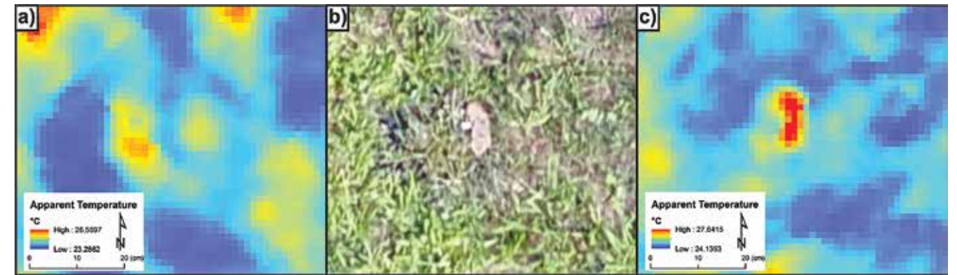
Figure 6. Apparent temperature from (a) 8:16-8:23 AM flight and (c) 9:18-9:24 AM flight before and after direct heating from sunlight, and (b) visible light color photos over the same area. Aluminum KSF-1 casing can be seen in the top left and PFM-1 landmine in the bottom right.
